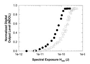
Figure 4. OECSFs of the G channel under spectral exposure series of  $\lambda = 550$  nm, varying internally t as 20 ms (solid circle), 10 ms (hollow square) and 5 ms (hollow triangle up) with the same f-number N = 2.8.
