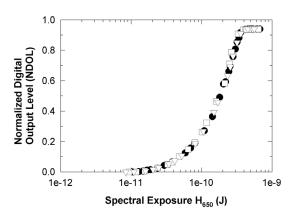
Figure 3. OECSFs of the R channel under spectral exposure series of  $\lambda = 650$  nm, varying N as 5.6 (solid circle), 4 (hollow square) and 2.8 (hollow triangle down) with the same shutter time  $t_0 = 20$  ms.
