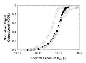
Figure 6. OECSFs of the B channel under spectral exposure series of  $\lambda = 450$  nm varying N and t to select two groups of three equivalent exposure series. First group: (hollow triangle up) for (N = 5.6, t = t<sub>o</sub>=20 ms), (solid triangle down) for (N = 4, t = 10 ms) and (x-hair squares) for (N = 2.8, t = 5 ms). Second group: (hollow triangle down) for (N = 4, t = t<sub>o</sub>=20 ms), (solid square) for (N = 2.8, t = 10 ms) and (x-hair circle) for (N = 2, t =5 ms).
