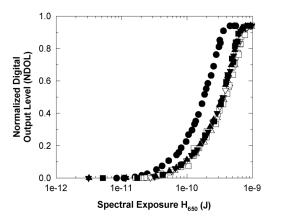
Figure 7. OECSFs of the R channel under spectral exposure series of  $\lambda = 650$  nm, varying t as 20 ms (solid circle), 19.9 ms (solid triangle up), 19.5 ms (solid triangle down), 17.5 ms (solid square), 15 ms (hollow triangle down), 10 ms (hollow triangle up) and 5 ms (hollow square) with the same f-number N = 2.8.
