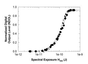
Figure 5. OECSFs of the G channel under spectral exposure series of  $\lambda = 550$  nm, varying externally t as 19 ms (solid circle), 38 ms (hollow square) and 76 ms (hollow triangle up) with the same f-number N = 5.6. The OECSF curve (solid diamond) with N = 4 and the internal shutter time t = 10 ms has been included.
