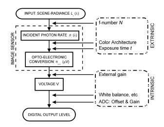
Figure 1. Scheme of the extrinsic and intrinsic parameters that can alter in a non-controlled and/or controlled way the raw optoelectronic conversion of a digital camera.
